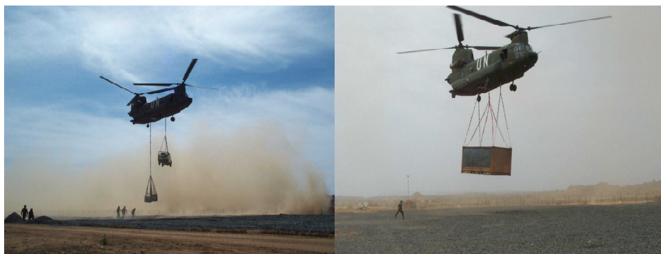
Fig. 1. Chinook helicopter transporting single and multiple loads (Courtesy of the Royal Netherlands Air Force)
